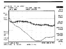
With the HP 11770A, the response of a coax cable can be measured between head-end and the subscriber output. This measurement will include the effects of amplifiers and frequency translators in the path.
