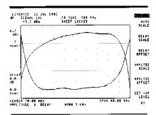
The quality of service available from a transmission network depends on the adjustment of the amplitude and group delay responses. Here we show the response of a digital microwave radio.
